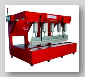
can be operated with hand or foot control. Bottom and top welding bars
