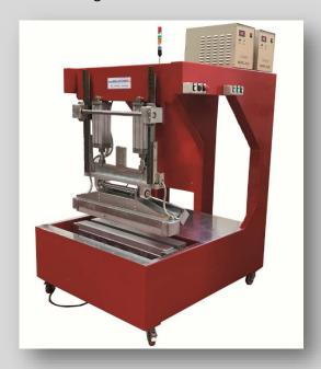
The BR10 PTFE welders are available in various size and for various purposes. This machine operates in two-step positioning mode that enables the precise placing of material and straight welding seam effectively avoiding the accidental seaming. Welding rod is usually 100x1000mm, but it could be upgraded according to client's demands. Special engraved electrodes are also available.
