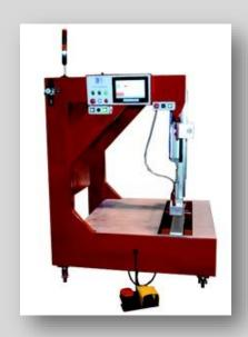
Balacchi's PTFE welding machine is easy to use, reliable and ergonomically friendly. Balacchi BR10PTFE can be easily moved thanks to strong wheels, which also facilitate the manipulation of the material during the welding process. Pneumatic cylinders lift up to 200mm that allow large-dimension roles to be used. Central control panel is intuitive and easy to use while the machine
